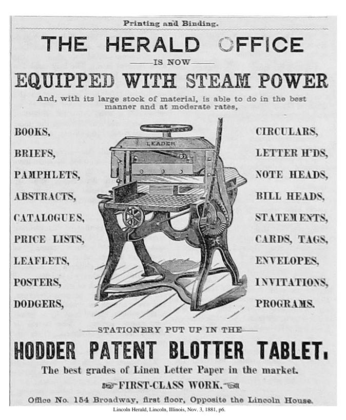
The piece of equipment shown here is a paper shear that was used to trim bound pages so they are the same width and length. With steam power heavy arm work and foot treadle work were eliminated.
